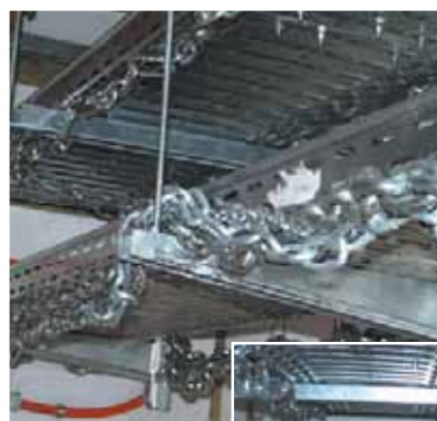
Chains applied as weight simulation.
