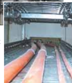
Chains applied as weight simulation.
